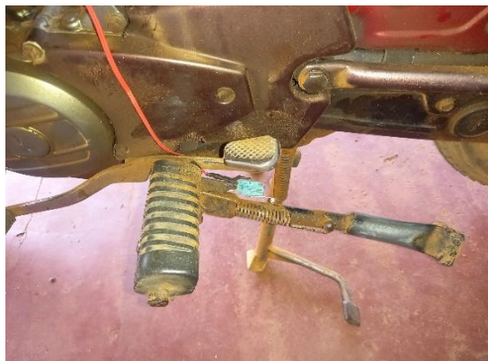
Figure 6. Arrangement to detect the position of side stand
