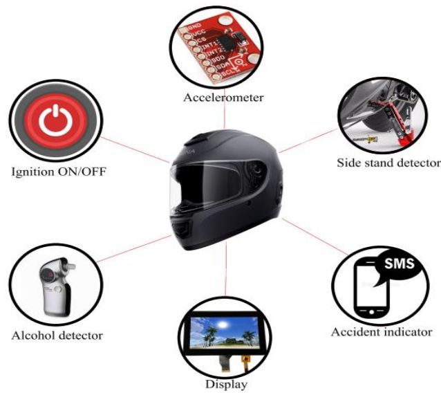
Figure 1. Integrated system of Smart Helmet
