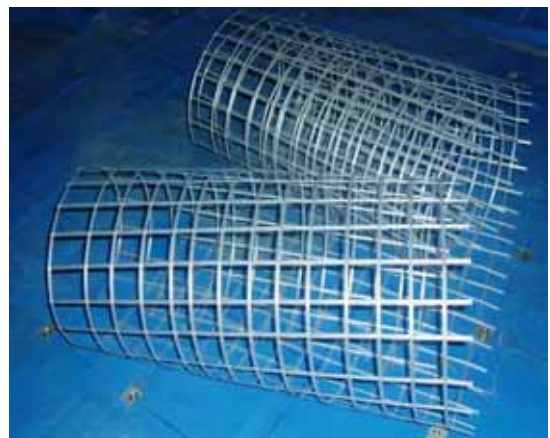
Figure 1 Polypropylene band mesh used for retrofitting
