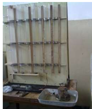
Figure 9: Hydraulic gradient apparatus
