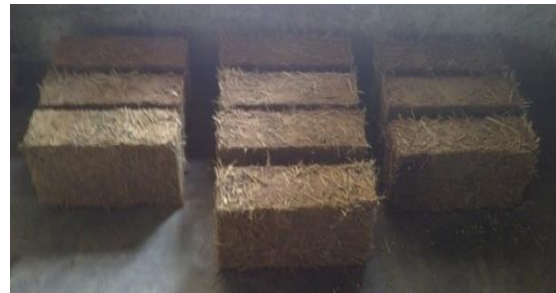
Figure 4: Casted, compacted mud block
