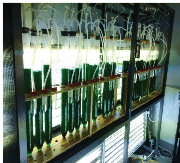
Fig. 1. Algal photo bioreactors used in the study
