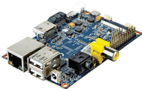
Fig. 5. The banana pi board of the base station [12].
