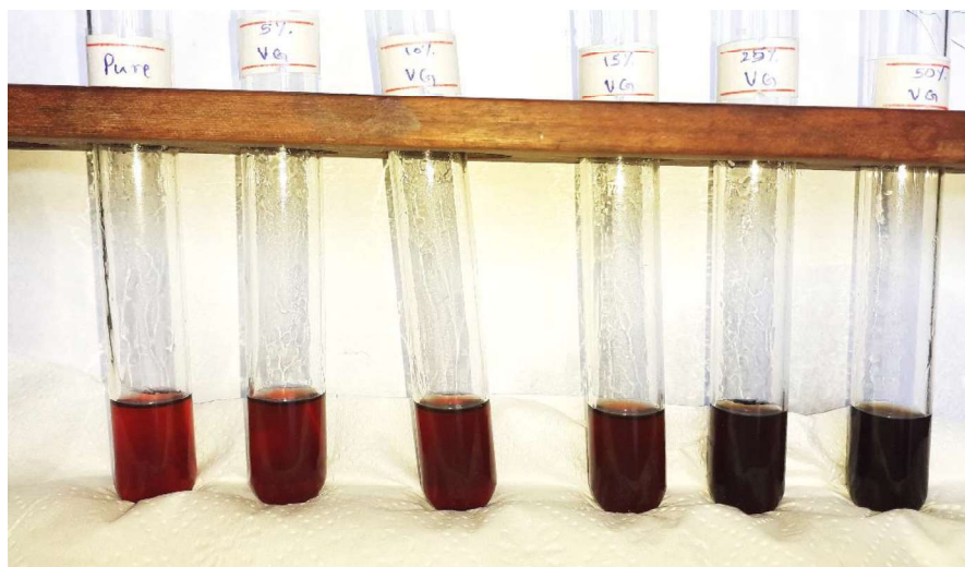
Figure 4: Modified Salkowski's test results of pure ghee adulterated with vegetable ghee (VG)
